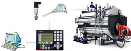
Process Boiler Control and Data logger Temp-Pressure
